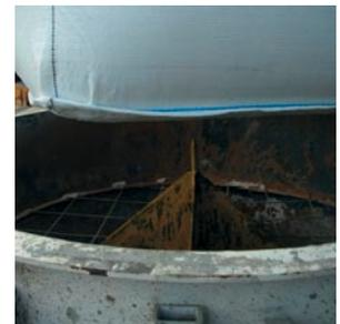
The bag is opened by cutting a cross in the bottom of the bag by using either a knife or an emptying device in which a knife and a screen are mounted.
